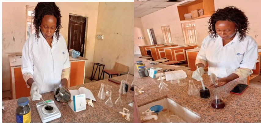
Plate 4: Weighing of activated carbon and stirring process of activated carbon plus abattoir effluent in a beaker
