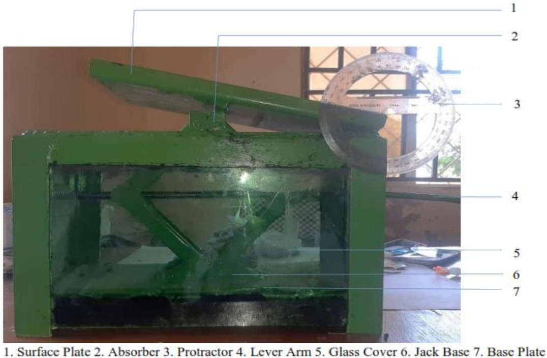
Figure 2: The Developed Coefficient of Friction Apparatus
