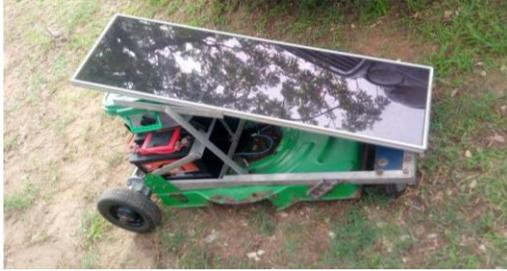
**Fig. 5: The Assembled lawnmower**
