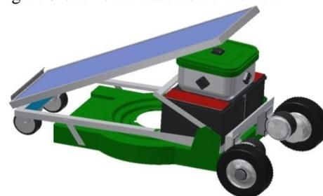
**Fig. 4: AutoCAD drawing of the Lawnmower**
